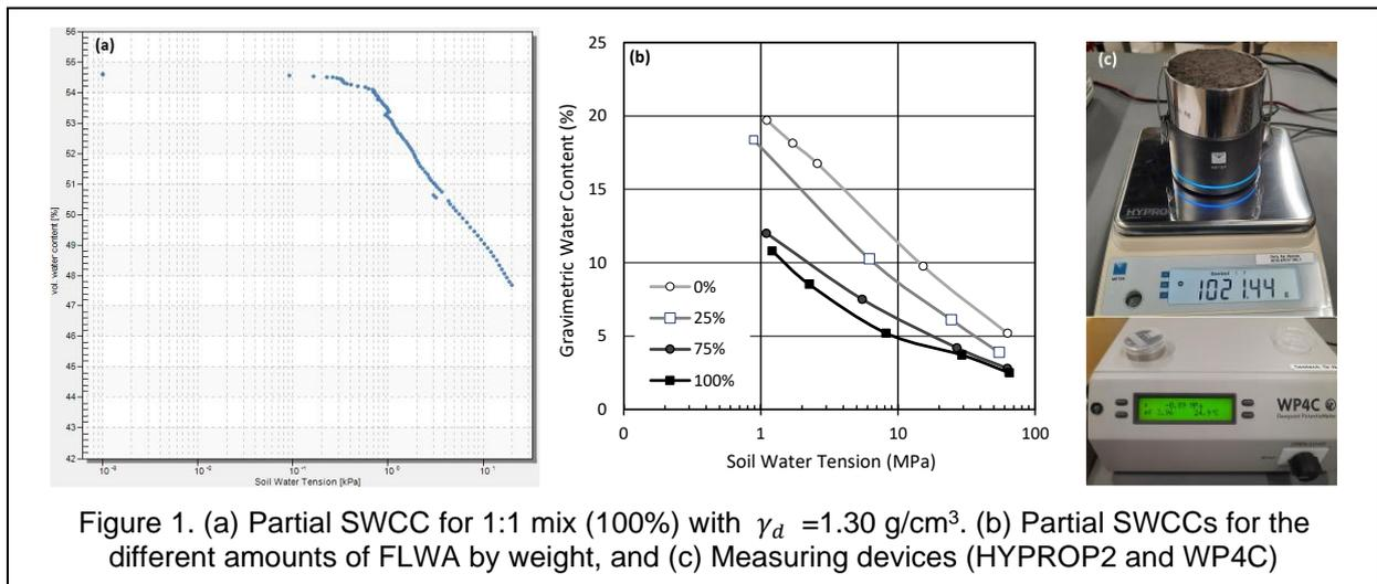
Figure 1. (a) Partial SWCC for 1:1 mix (100%) with  $\gamma_d = 1.30 \text{ g/cm}^3$ . (b) Partial SWCCs for the different amounts of FLWA by weight, and (c) Measuring devices (HYPROP2 and WP4C)
